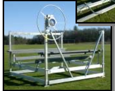
Model MH-V45108 with carpeted guideons and motor stop
