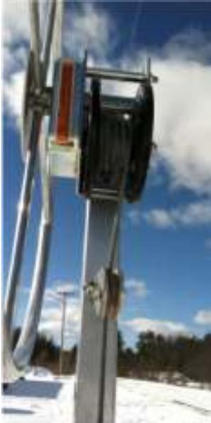
(24/1-5) Install the cable clamp assembly using the square hole on the side of the winch. Only thread nut on just far enough to prevent clamp from coming off. Put free end of cable thru hole in side of winch below the clamp, push cable thru one side of the clamp, make a large loop then push cable back thru the other side of the clamp. Carefully pull the loop out as shown in step 4. Leave the end about 1" beyond the clamp then tighten securely.
