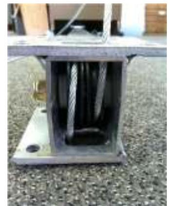
View of rear Beam with (2) cable/sheaves pre-installed. Front Beam will have only one.
