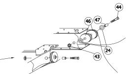
EXPLODED VIEW OF SHEAVE ASSEMBLIES LOCATED IN REAR TWIN BEAM AND CRADLE TUBE LEFT OR RIGHT
