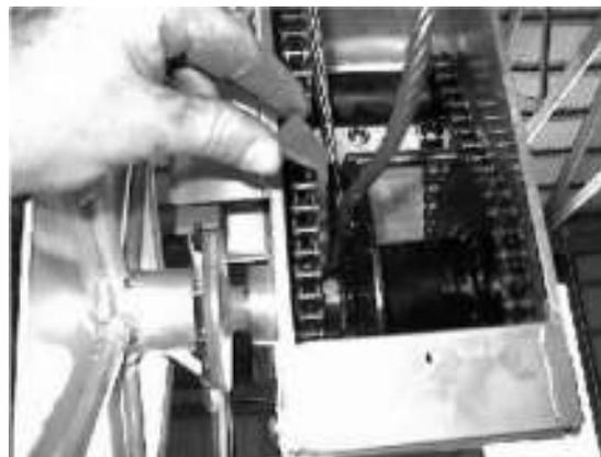
Place the cable wedge in the loop then pull cable tight and lock wedge in tight cable loop
