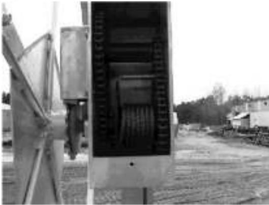
Winch bolted to hoist with wheel assembled. Cable goes through bottom of winch.
