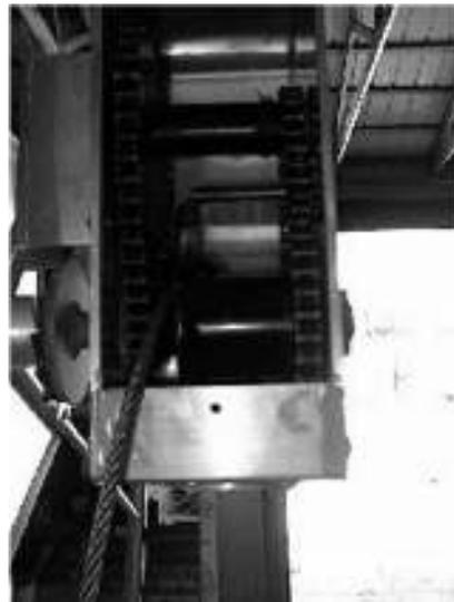
Pull cable out and make a loop and put the end of the cable in the cable holder on the outside of the spool.
