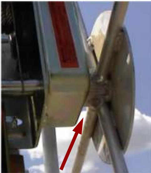
(22) Thread the 30" wheel on the winch shaft as far as it will go making sure it's tight against the winch, when the wheel makes contact on winch brake pad you will hear a clicking noise when wheel turns clockwise.
