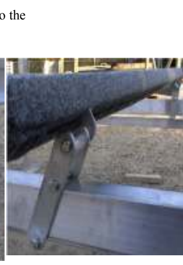
Carpeted bunk board mounted on bunk bracket assembly.
