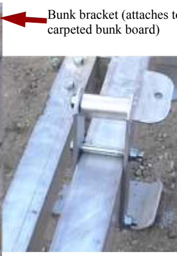
Bunk bracket assembly mounted on lift beam.
