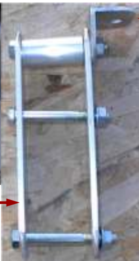
Completed bunk bracket assembly
